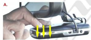
5 - To access the buttons of the RD you will need to gently push downward on the front of the RD with one finger and push the desired button with another finger (fig A.). Then allow the RD to return to it's original position by gently letting it spring upward. When accessing the buttons, be sure to push the RD downward just enough for your finger to fit between the RD and mirror.
