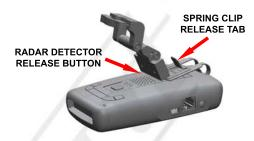
2 - Push the RD release button when installing and removing the RD onto the spring clip. Slide the clip into the RD as far as possible. Install the RD a few times so you can observe how the spring clip functions. When used properly, the spring clip avoids putting excessive pressure on the mirror stem when installing and removing the RD.
